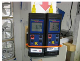
Fig. 4. Temperature monitors showing manikin input air temperature and manikin output air temperature values which are needed to compute manikin heat loss values.
